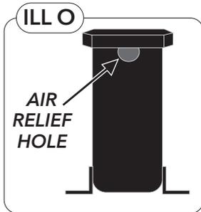
2. While filling with concrete, gently tap on the very center of the top of the base with a block of wood or handle end of a hammer.
